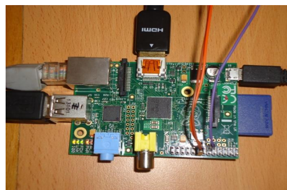
Fig.2.1.2 Connections to Raspberry Pi
